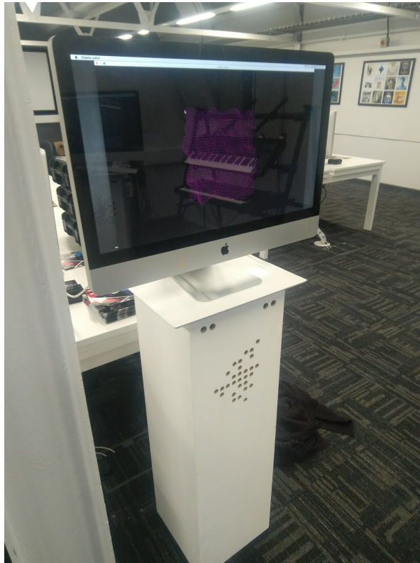
Fig 15 - iMac on top of a plinth. Inside there are two ultrasonic distance sensors and a speaker.
